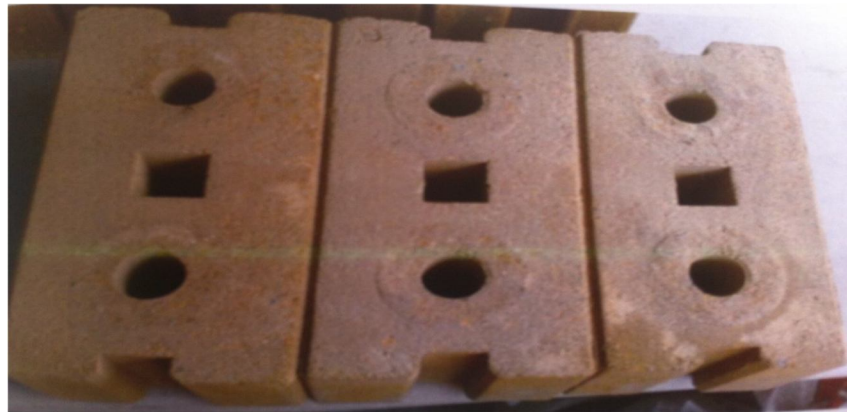
Fig (3) Flatted surface of Soil –cement interlocking brick without mortar fill
